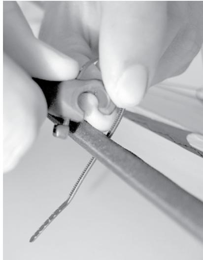
Figure 3: Yo-yo fitting installation
